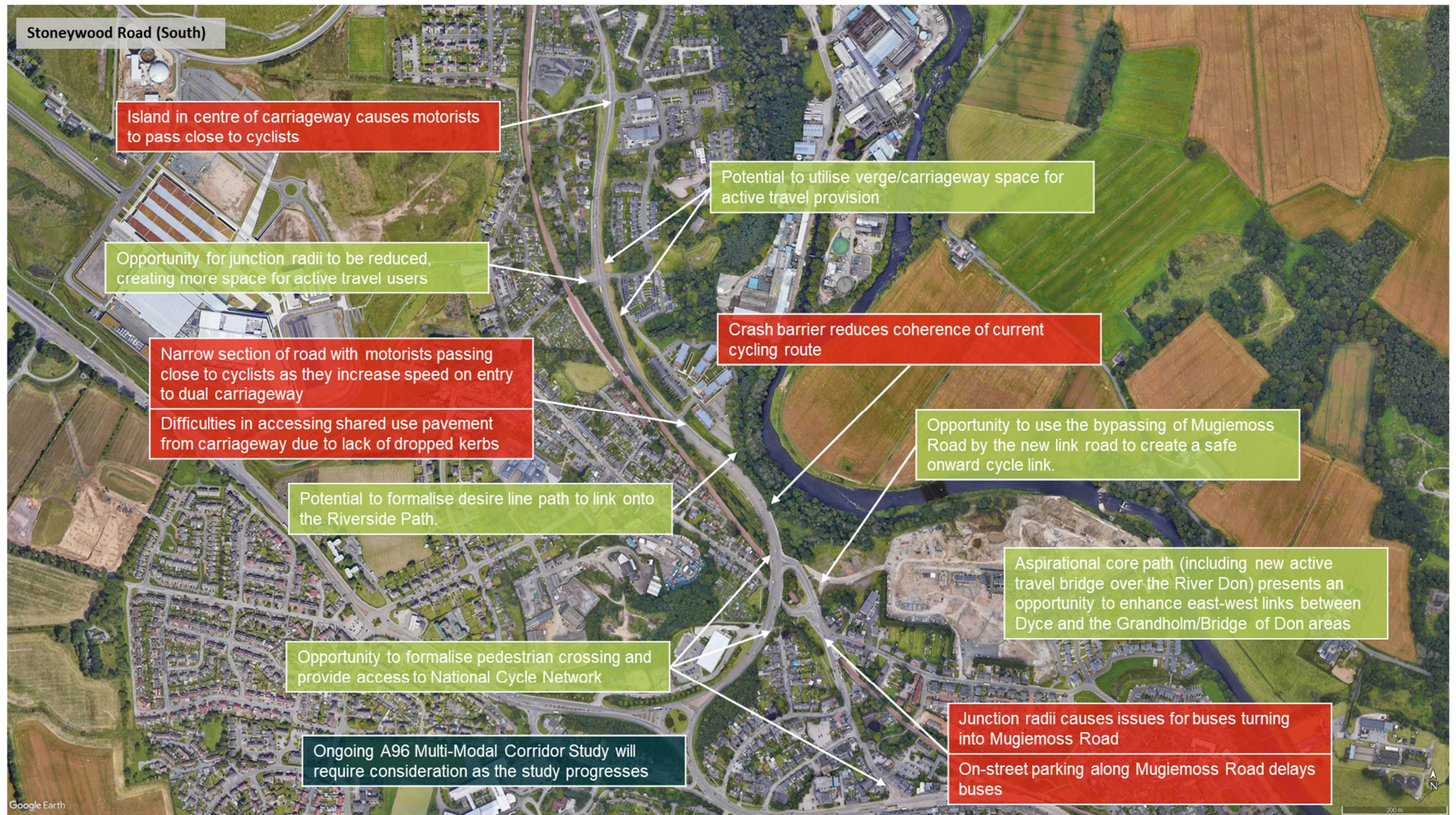
Figure 4.10: Location-Specific Issues on Stoneywood Road (South) (Image Source: Google Earth)
