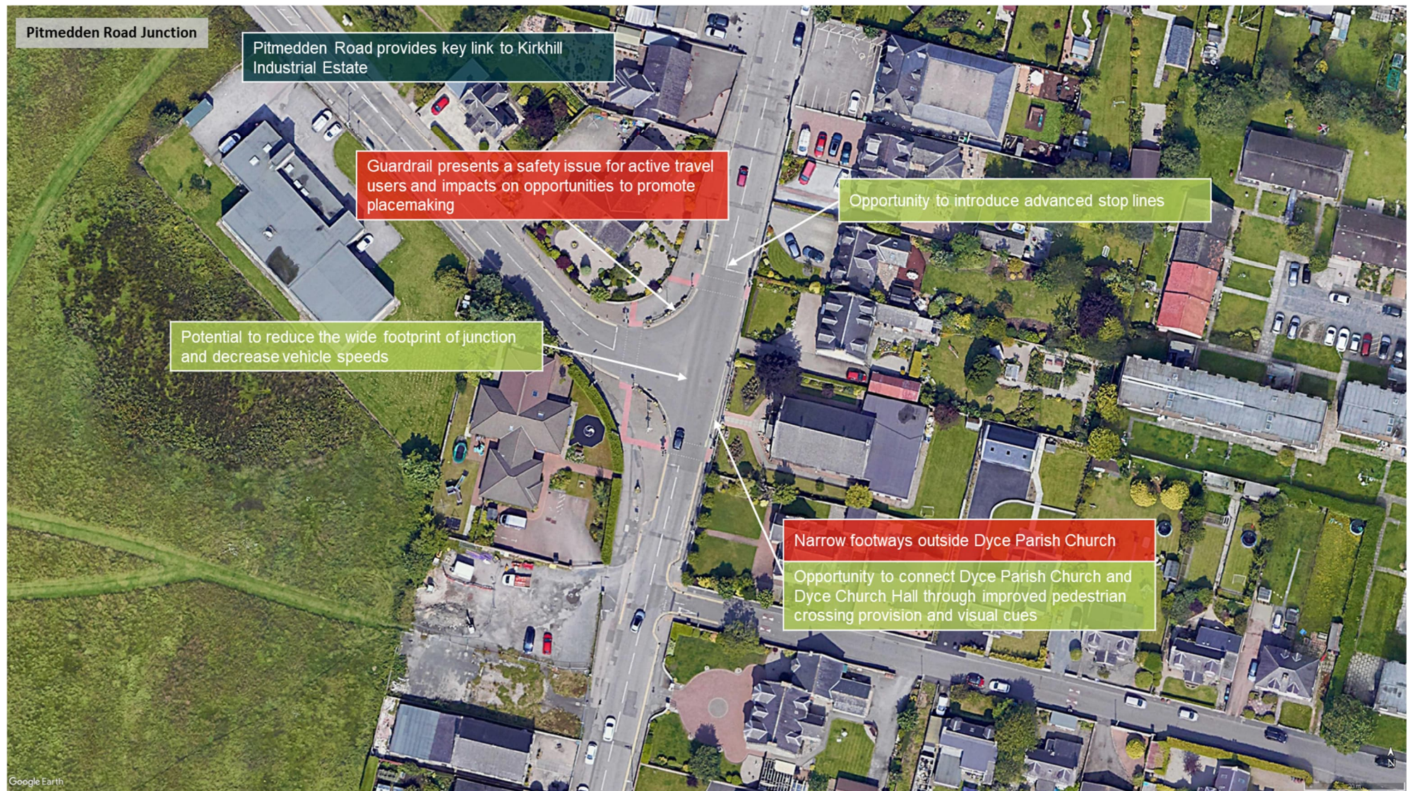
Figure 4.6: Location-Specific Issues at the Pitmedden Road Junction (Image Source: Google Earth)
